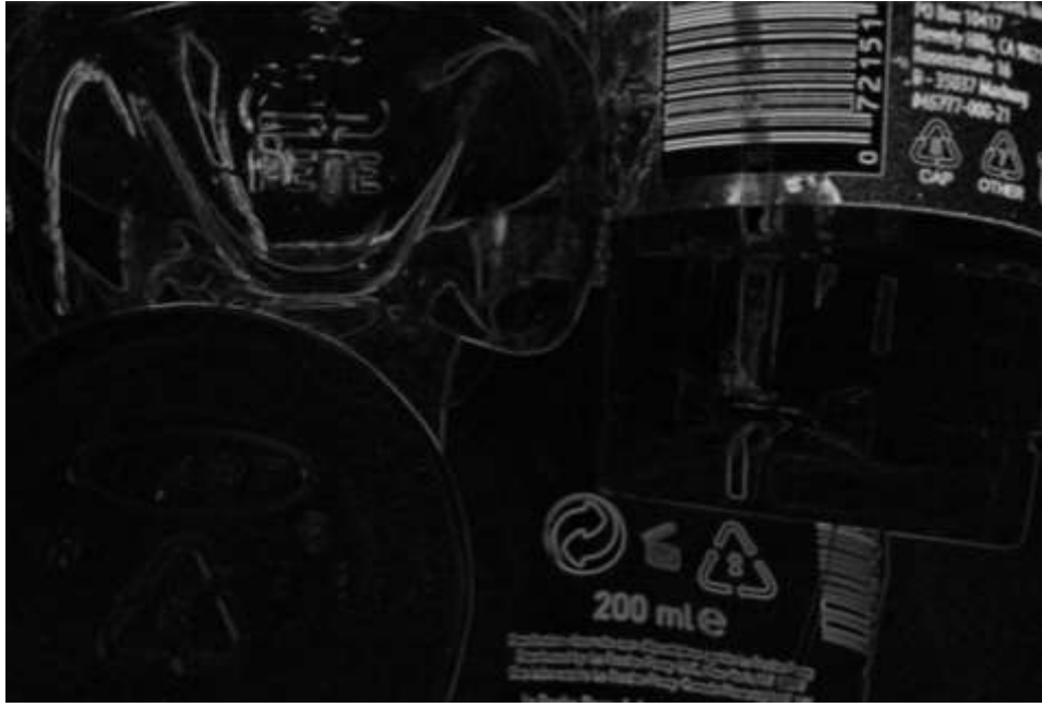
Fig. 6 – Result of applying the Sobel operator to the image
